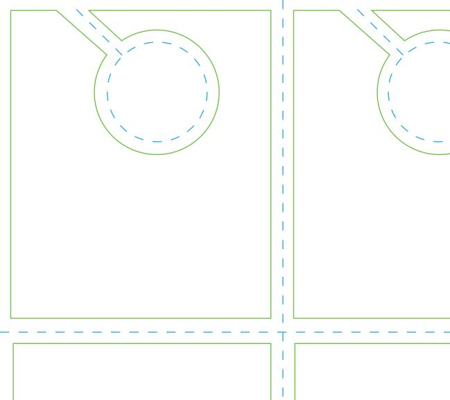
Green Lines indicate "Safe Print" area. For best results keep printing 1/8" away from perforations, edges and folds.
