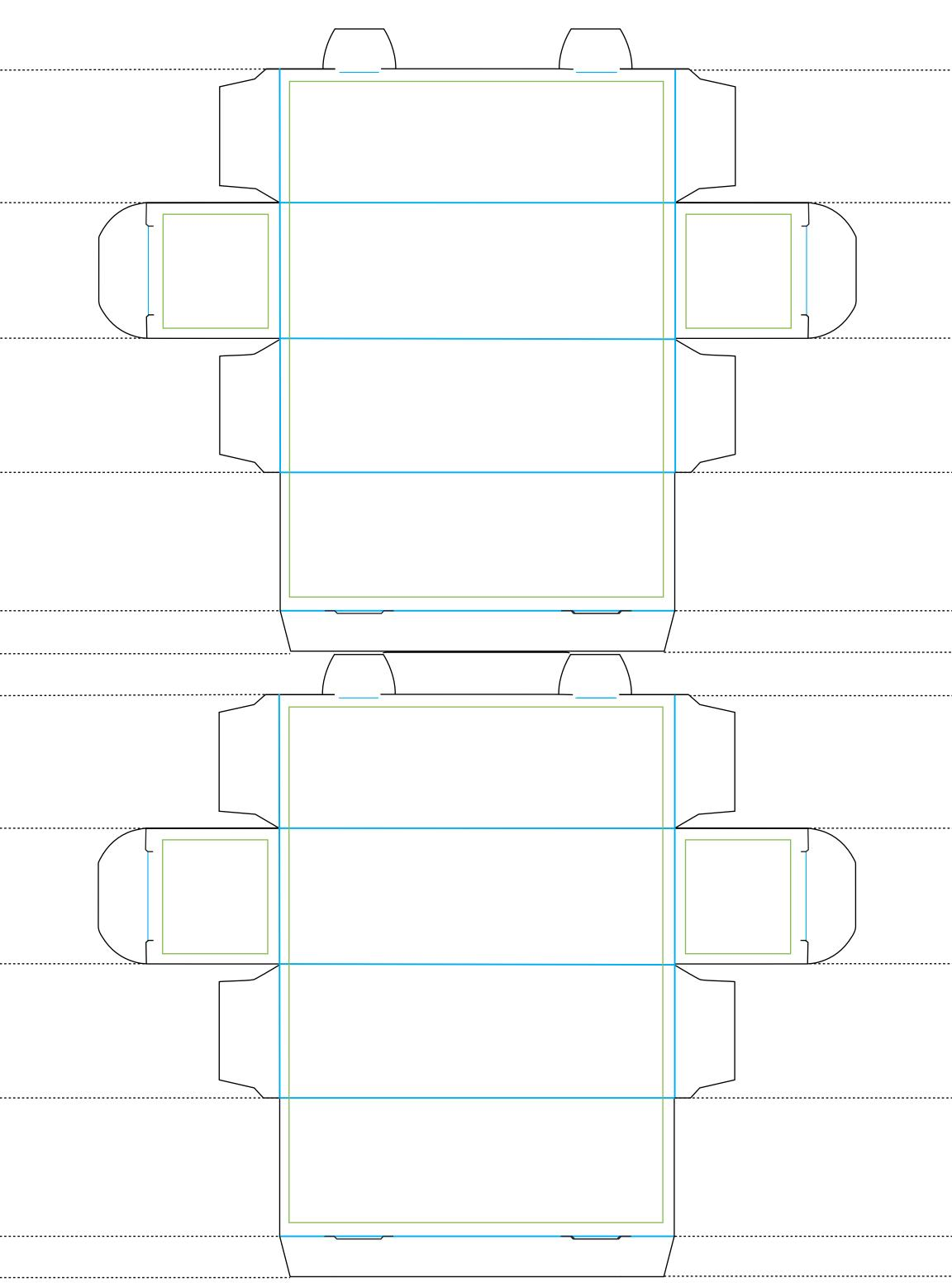
Green Lines indicate "Safe Print" area. For best results keep printing 1/8" away from perforations, edges and folds.
